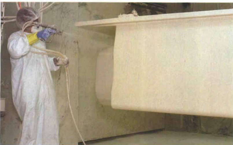
First stop on the production line is a gelcoat spray booth where the mold is sprayed with an initial coat of resin. In later steps, chopped fiberglass twine is mixed with polyester resin to build wall thickness.
